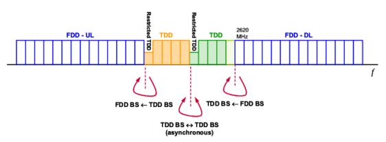
This restriction is due to the need to ensure suitable technical conditions for the coexistence of systems using frequencies in adjacent blocks serving for unlimited TDD and FDD traffic, or – in the case of two unsynchronised networks operating in the TDD mode – to ensure the compatibility defined in Commission Decision  $2008/477/EC^{26}$ . D1 segment restriction will not be applied where the same Applicant becomes the Holder of the Allocation of the segments D1 and C14.
